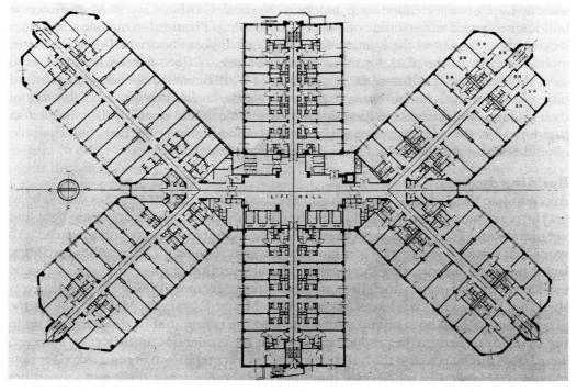
Fig. 8 White House, Regent's Park, London. Plan of a typical upper floor. Architect & Building News, 1936.
